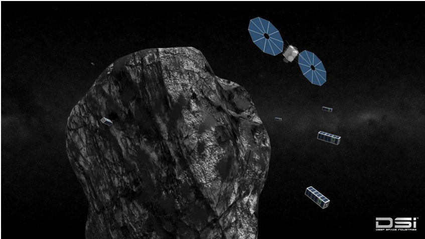
Figure III.2 The Mothership of Asteroid CubeSats offered by DSI delivers multiple low-cost CubeSats for joint investigations of NEA targets.
