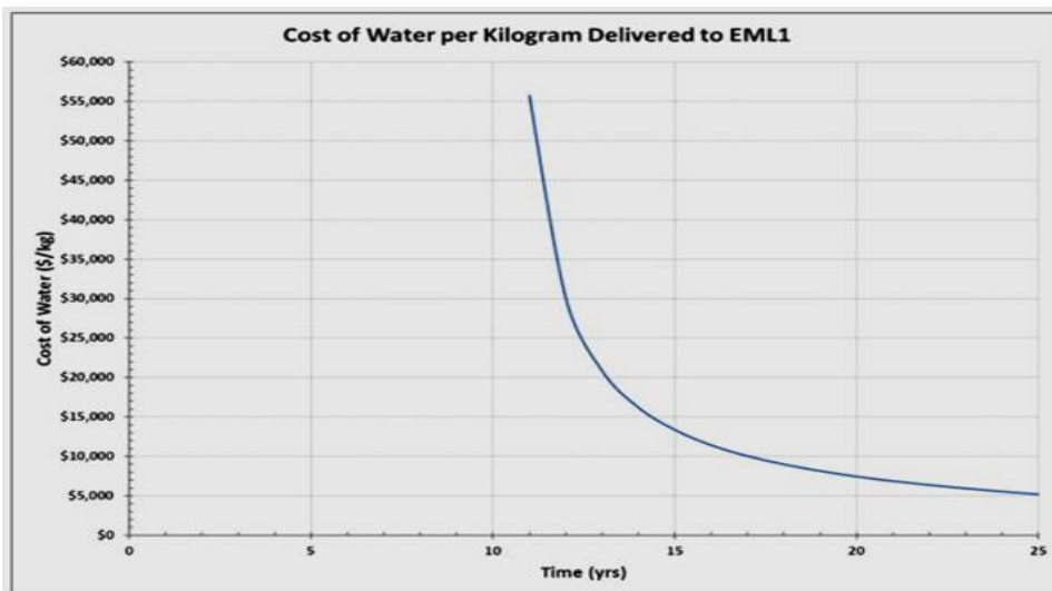
Figure 7.14. Unit cost of water delivery to EML-1 for RAP architecture [Cohen, 2013b].
